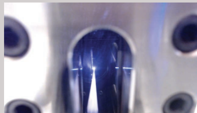
Pulsed laser beam entering high-pressure superficial carbon dioxide. The plasma formed produces nanoparticles for catalysis.
